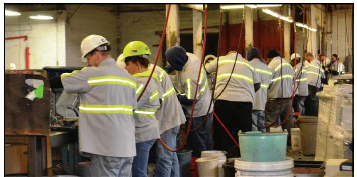
Workers at Cohen’s E-Waste Division use pneumatic screwdrivers to disassemble computers and other electronics.
